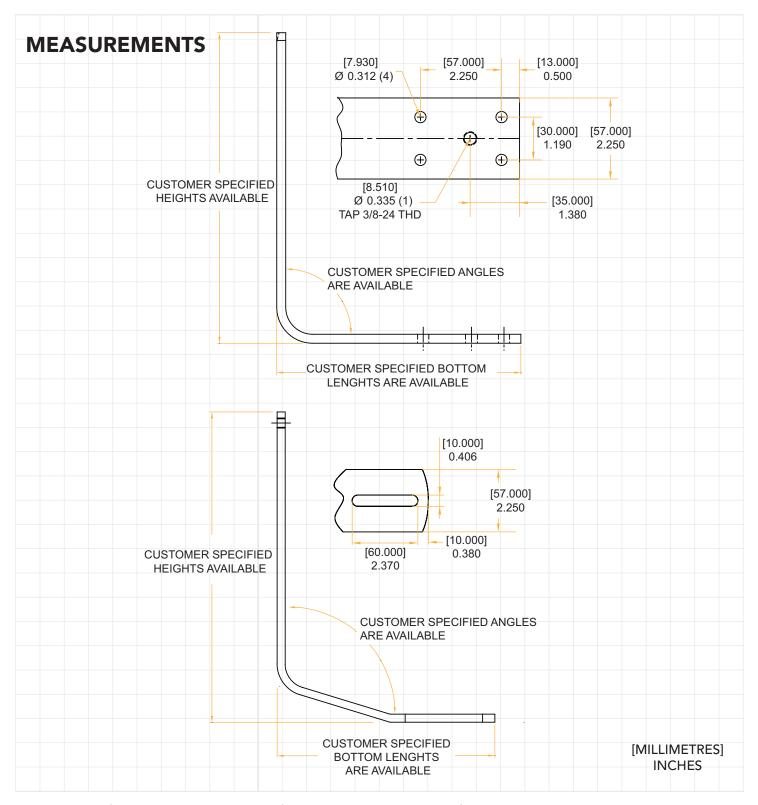
NOTE: A variety of bottom hole patterns and slot configurations are available. Custom configurations may require tooling.
